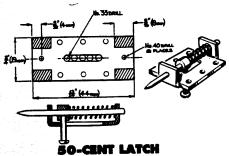
You'll need a 3/4x19/4-inch piece of 1/1e-inch (1.5mm) aluminum, a 3/52-inch (2mm) wire pin, a matching wheel collar and a no. 20 spring from a hardware store. Cut out the shaded areas with a saw, drill holes where shown and bend up the two end tabs. Use epoxy or screws to mount the latch on the hatch or canopy. You could also use a piece of U-shaped channel aluminum to avoid having to bend the sheet aluminum.
