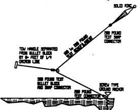
this type of setup, make sure that the anchored end of the line is attached to a stake that will not pull out of the ground and become a missile. The typical high-start stake will not do. Use a screw type aircraft holddown, or a stake which can be driven into the ground at least 18 inches. Your tow-man will be standing very close to this stake at the beginning of the tow, and the force on the stake can approach the breaking strength of your tow line. Should the stake come
