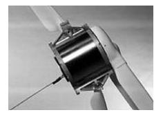
A close-up of the motor showing its very simple mechanical design. The hinged propellor blades are attached directly to the outside rotor, the inside stator is fixed to the pylon and a cable pulls the assembly into the fuse for soaring. I figure three
